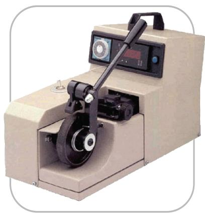
It is used to measure the force - expressed in Newton - needed to pull a terminal off a crimped wire. The pulling speed can be set beetween 15 and 120mm/min is about 4.7 in/min. The instrument has a serial communications port. Every SMST is tuned in our laboratory, and its calibration is carried out with Mecal specific equipment MST 0158, fitted with 546 QDT force analyzer. Also available as splice version.
